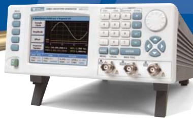
The sequence generator has four advanced modes: automatic, stepped, single and mixed, which make it even a more powerful tool.
