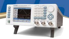
The sequence generator has four advanced modes: automatic, stepped, single and mixed, which make it even a more powerful tool.
